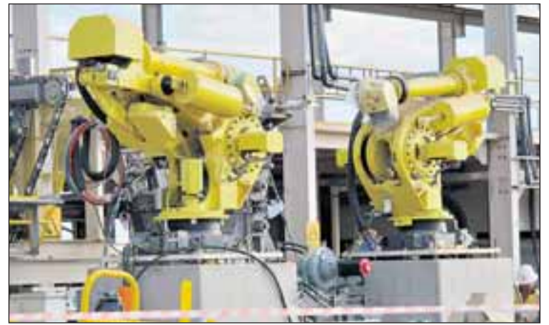
Lady Annie's two new 600kg payload robots have patented end-of-arm tooling for cathode plate handling and stripping which gives them a capacity of 150 cathode plates per hour.
